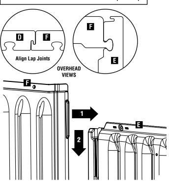
Engage snaps on bottom of Right Back (F) into Repeat Floor (B).
